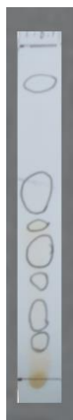
Figure 1. Chromatogram of the ethyl acetate fraction of ketapang fruit pulp with ethyl acetate : chloroform: glacial acetic acid (1:8:1) as eluent
