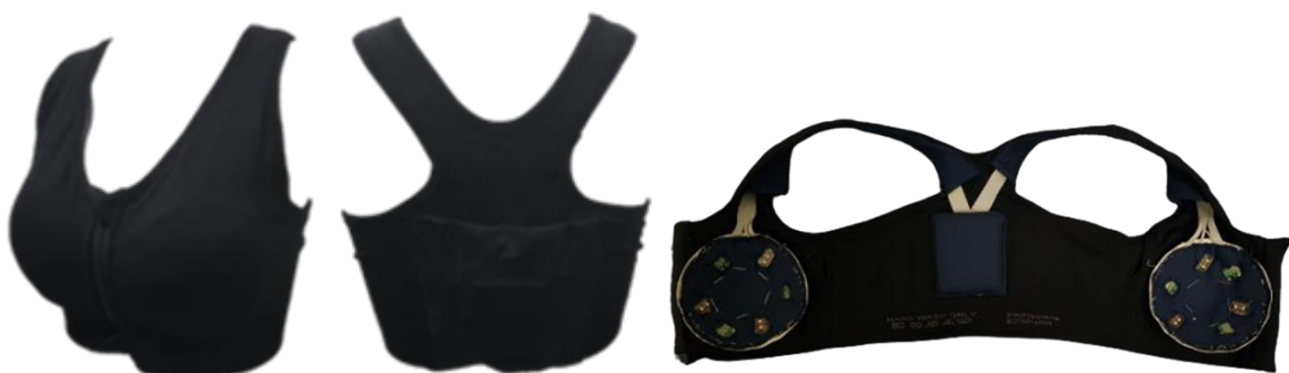
Fig. 9. Design of Smart Bra and Installation of the sensor on the bra cup and the controller module board on the back of the bra
