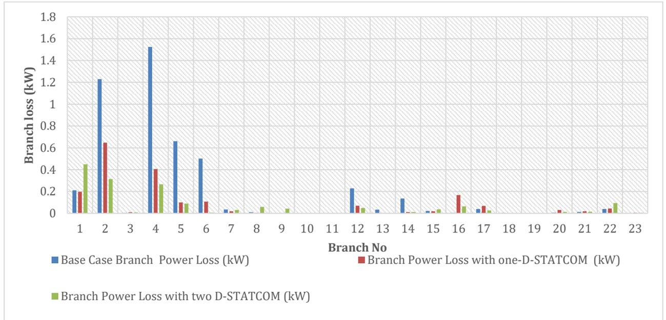
Fig. 11. Comparison of the profile of branch active power loss
