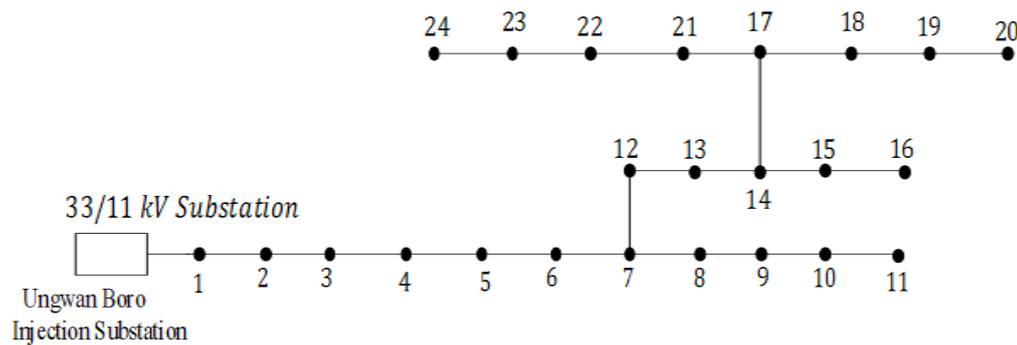
Fig. 2. One-line diagram of Pama 11kV, 24-bus RDN
