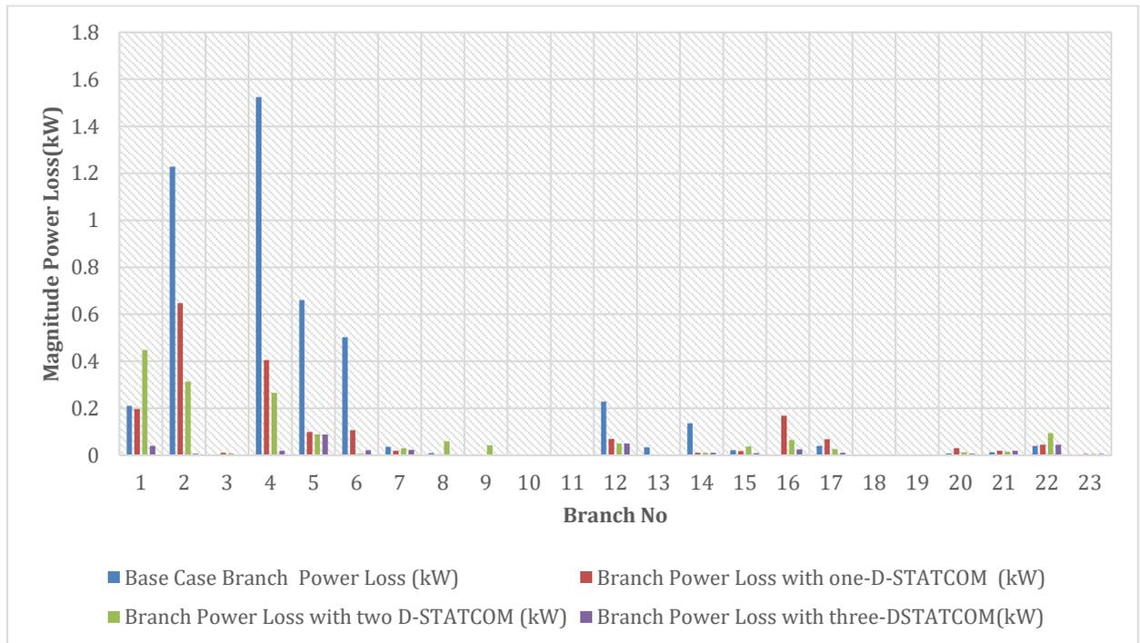
Fig. 14. Comparison of branch power loss profile
