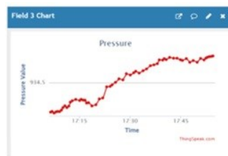
(c) Thingspeak visualization of pressure at February, 29 2024 in the period time 17.10-17.50 WIB (left). The value of pressure in the last point (right)
