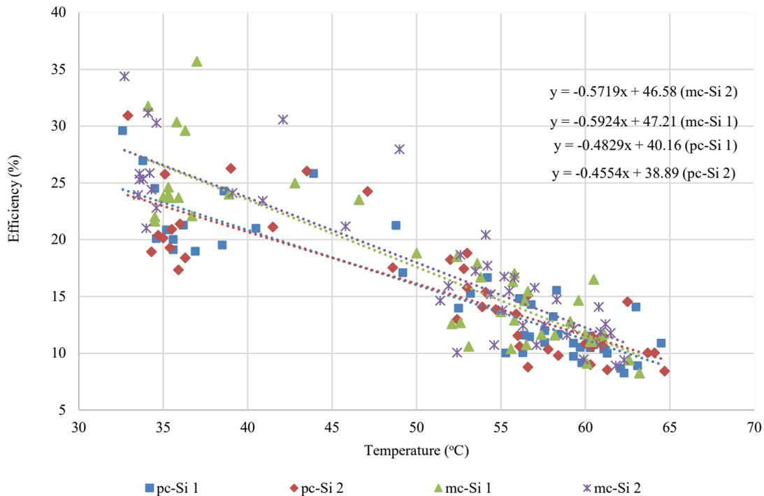
**Fig. 8.** Efficiency of PV modules without vegetation at different temperatures
