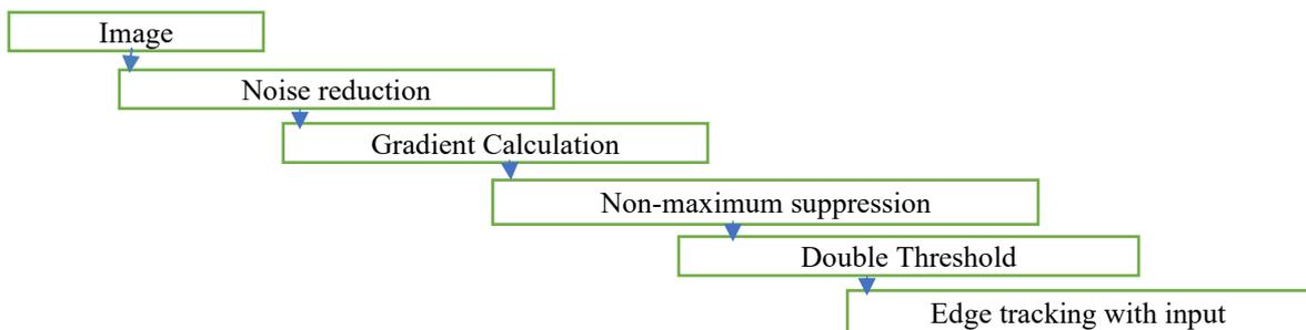
**Fig. 3.** Canny Algorithm Method
