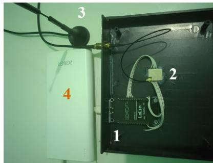
**Fig. 8.** Gateway (LoRa-Rx); (1) ESP32, (2) LoRa RA-02, (3) Antenna, (4) Powerbank.**Table 3.** LoRa-ESP32 pin configuration
