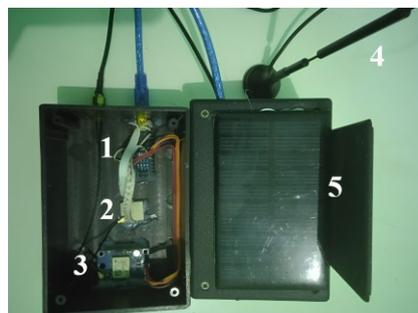
**Fig. 7.** Node (LoRa-Tx); (1) Board Arduino nano, (2) LoRa RA-02, (3) GPS UBlox Neo 6M, (4) Antena, (5) mini solar cell with modulator and battery.
