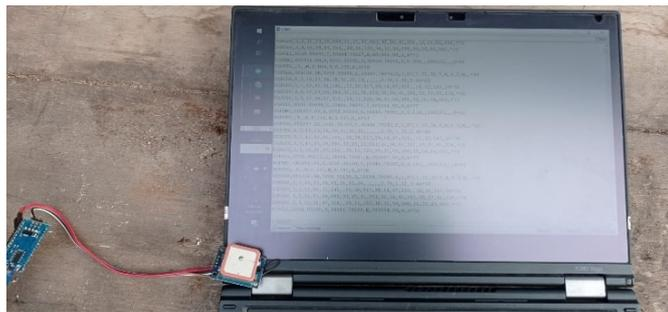
**Fig. 9.** Preparation of the GPS module connected to the PC in order to display NMEA messages through serial monitoring Arduino IDE
