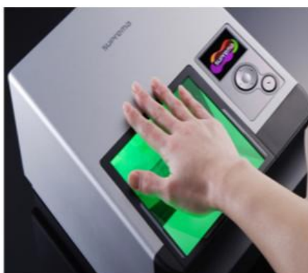
Fig. 2. Palm Print scanning process using scanner
