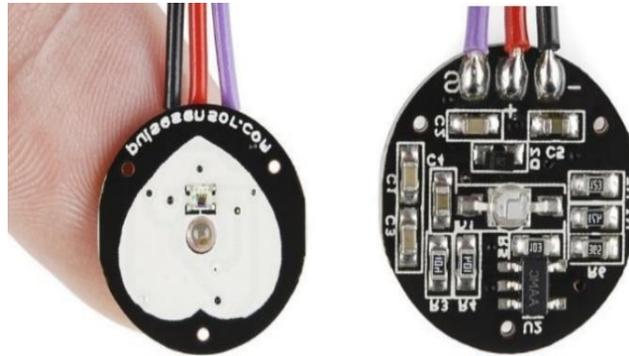
Fig. 4. Top view of the heart rate sensor
