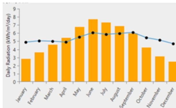
**Fig. 2.** Daily radiation ( $\text{Kwh/m}^2/\text{day}$ ) for the studied site
