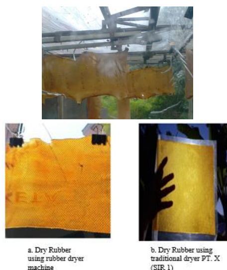
Fig. 11 Quality result testing of dry rubber
