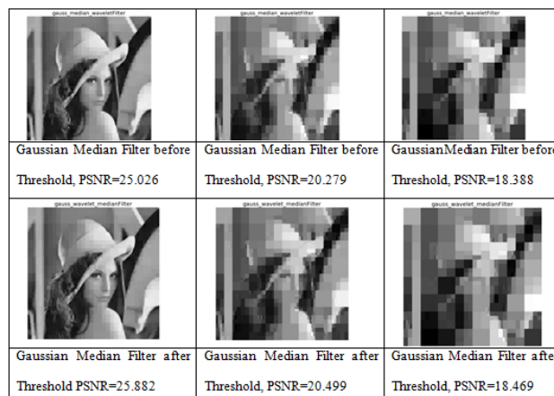
Fig. 7. Result of the PSNR value on de-nosing Lena image by median filter before and after threshold, noisy image corrupted by noise ratio=10,50,100
