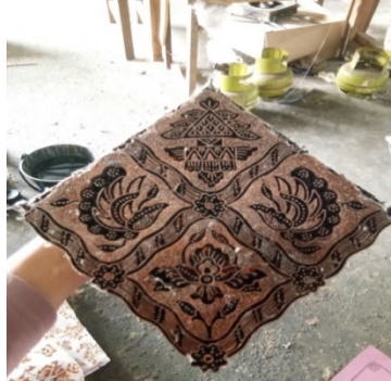
Figure 16. Stamps Used to Make Batik Sidoluhur
