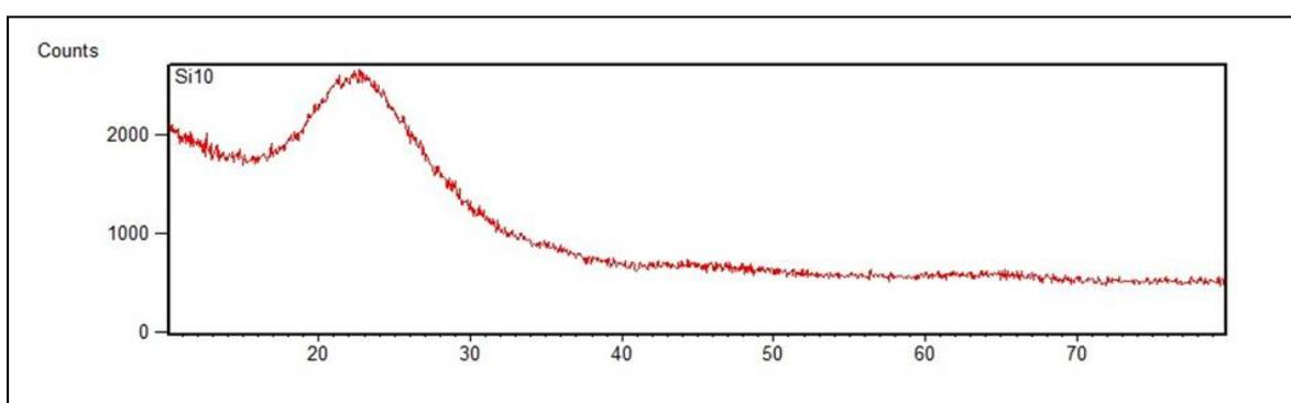
**Fig. 3.** X-ray diffraction of silica sludge
