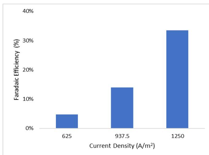
**Fig. 6.** Effect of the current density on the faradaic yield in the electrolysis of sodium silicate at  $3.3\text{ mol/L}$  NaOH and  $1/1\text{ g/mL}$  of solid/liquid for 2 hours at  $30\text{ }^\circ\text{C}$
