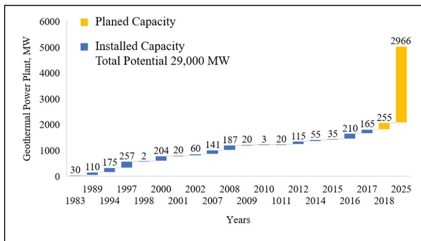
**Fig. 1.** Generation from Indonesian geothermal power plants: past, present, and future [6]
