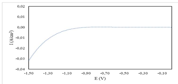
Fig. 5. Cyclic voltammetry in sodium silicate with  $3.3 \text{ mol/L NaOH}$  solution at  $30 \text{ }^\circ\text{C}$
