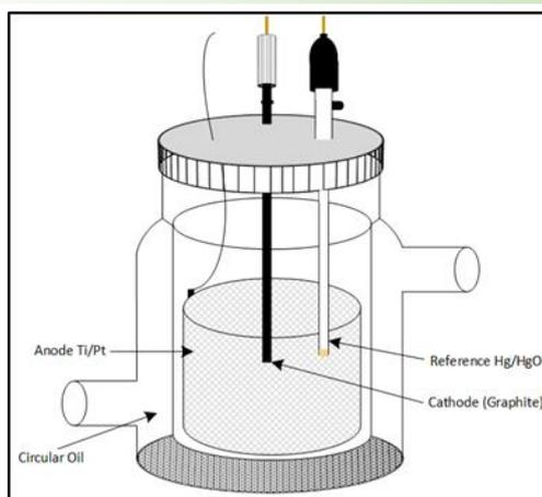
Fig. 4. Electrochemical cell
