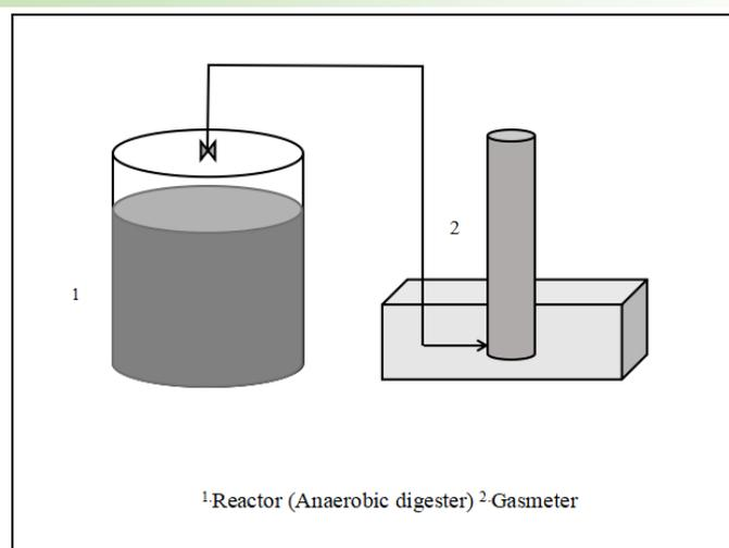
Fig. 1. Reactor and Gasmeter
