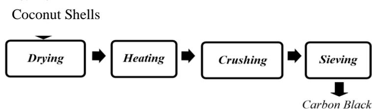
Fig. 1. Carbon Black Production from Coconut Shells
