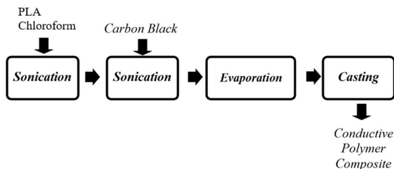
**Fig. 3.** Synthetic Scheme of Conductive Polymer Composite via Solvent Blending Method
