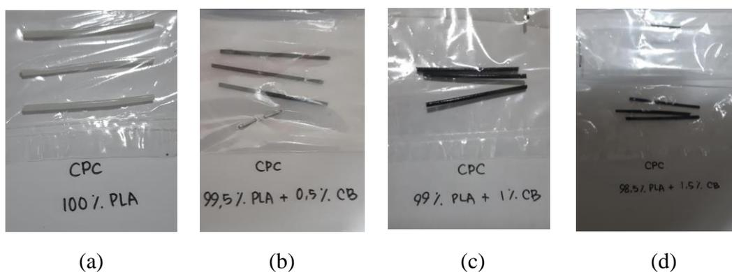
Fig. 5. Samples Prepared via Melt Blending with various CB compositions; (a) MPLA0 (b) MPLA05 (c) MPLA10 (d) MPLA15
