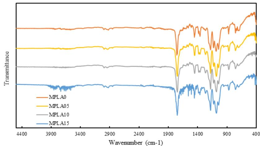
**Fig. 7.** ATR-FTIR of Samples Prepared via Melt Blending
