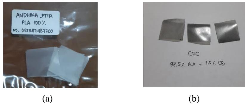
**Fig. 6.** Samples Prepared via Solvent Blending with Various CB compositions: (a) SPLA0 (b) SPLA15
