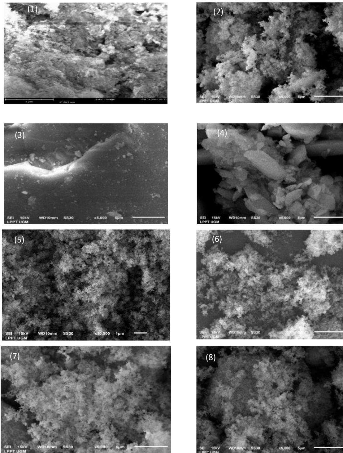
**Fig.5.** The surface morphology of SEM images: Silica before (1) and after (2) adsorption, Standard silica before (3) and after (4) adsorption, Mesoporous silica (MS1) before (5) and after (6) adsorption, (7) MS2 after adsorption, and (8) MS3 after adsorption
