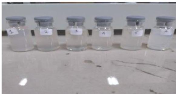
**Fig.3.** Adsorption of wastewater process: (1) printing waste, (2) adsorption silica, (3) standard silica, (4) MS 1 gr, (5), MS 2 gr, and (6) MS 3 gr
