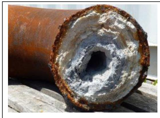
**Fig. 2.** After applying acidification to avoid silica scaling, a pipe at the Dieng Geothermal Power Plant became clogged.
