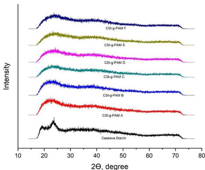
Fig. 2. XRD spectra between cassava starch and CSt-g-PAM
