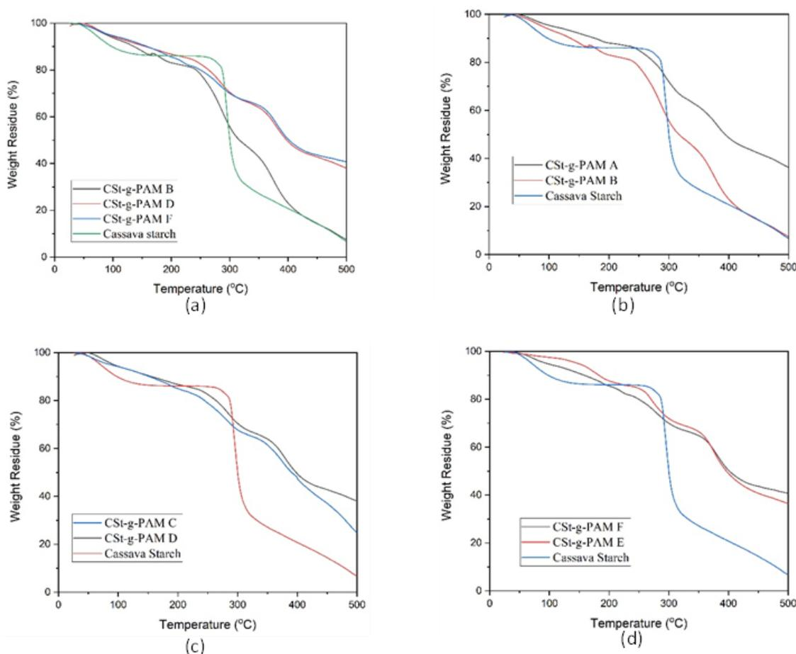
**Fig. 3.** TGA analysis of cassava starch and CSt-g-PAM (a) effect of acrylamide concentration (b) effect of time irradiation when acrylamide was 2 g (c) effect of time irradiation when acrylamide was 5 g (d) effect of time irradiation when acrylamide was 10 g
