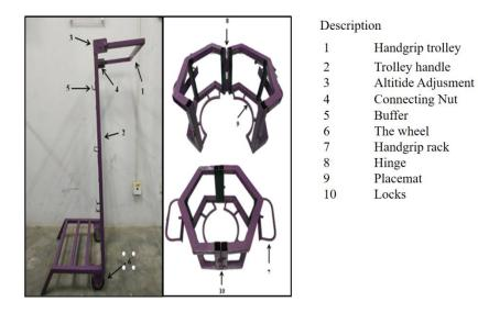
Figure 3. An Ergonomic Trolley for Handling Task
