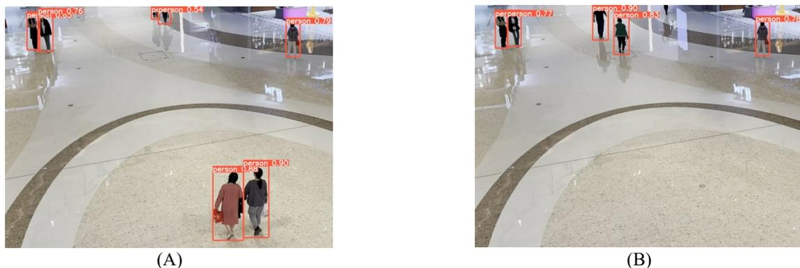
Fig. 9. (A) Human Detection 100% correct (B) Human detection error
