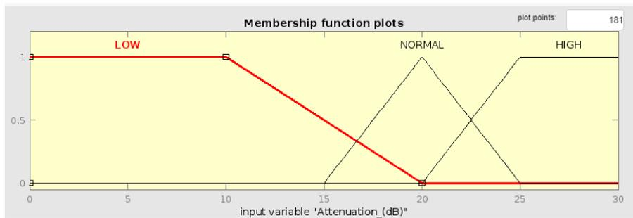
**Fig. 5.** Membership Function Variable "Attenuation"
