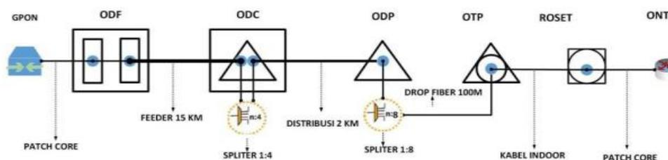
Fig. 2. Architecture and Topology of GPON [6]
