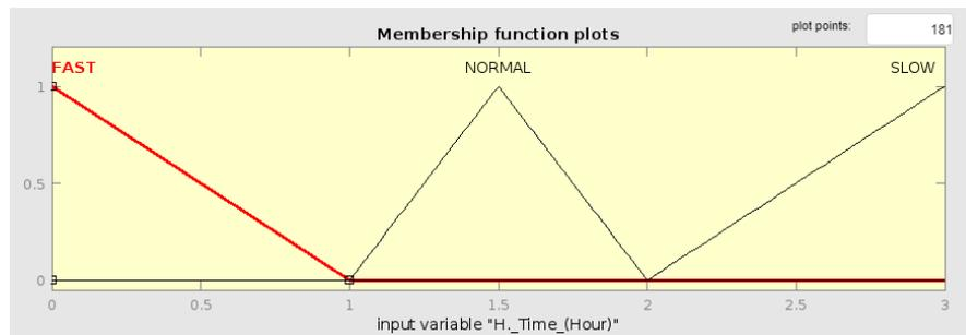
**Fig. 4.** Membership Function Variable "Handling Time"
