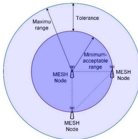
Fig. 10. Acceptable Wi-Fi signal tolerance
