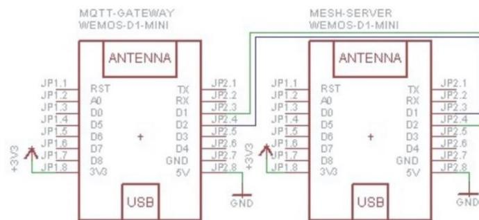
**Fig. 5.** Schematic of gateway circuit
