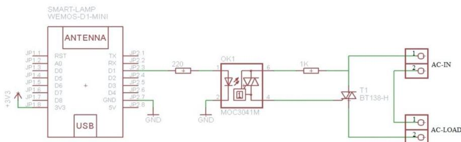
**Fig. 3.** Schematic of the smart lamp circuit
