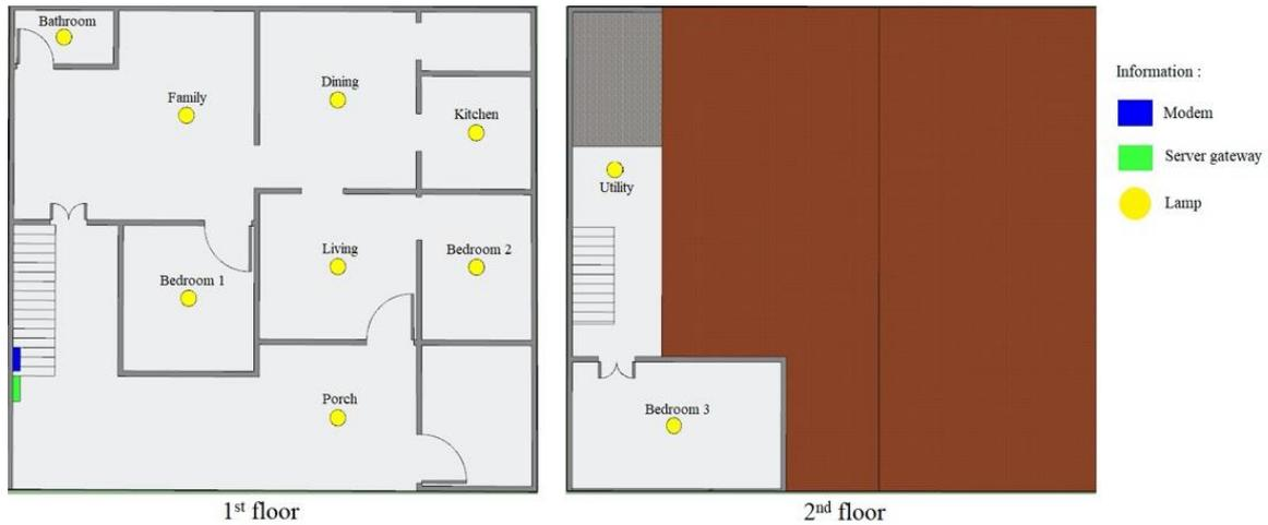
Fig. 9. The layout of the lamp placement
