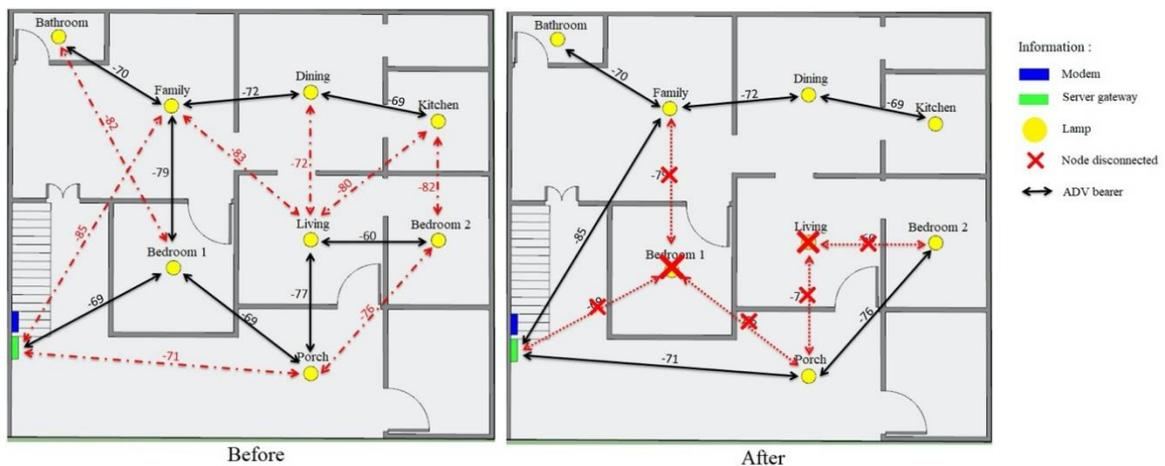
**Fig. 13.** Disconnected path due to two disconnected light nodes
