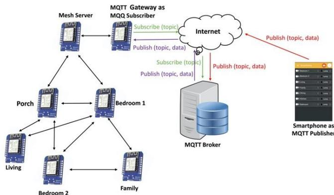
**Fig 6.** Working as an MQTT broker in the smart light system
