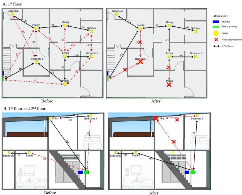
Fig. 15. Disconnected path due to 3 disconnected light nodes
