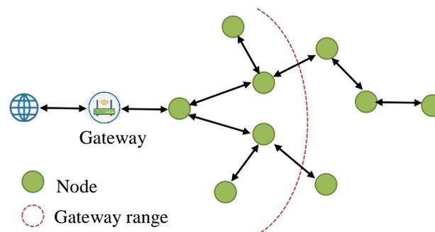
**Fig. 1.** Multi-hop ESP-Mesh network topology
