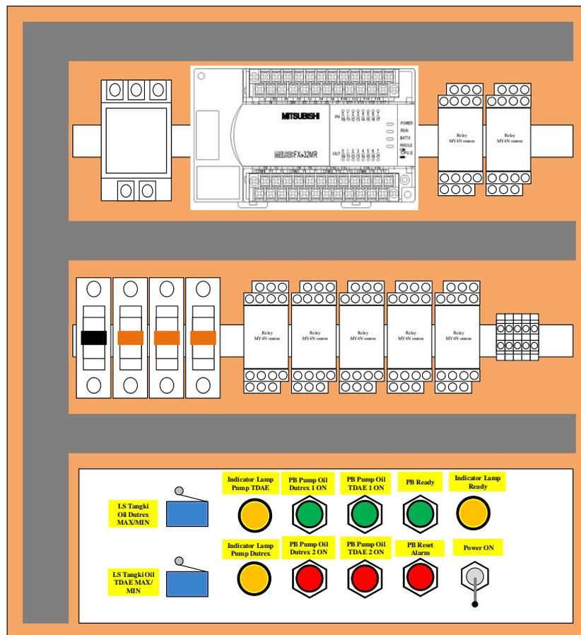
**Fig. 4.** Control Panel Layout
