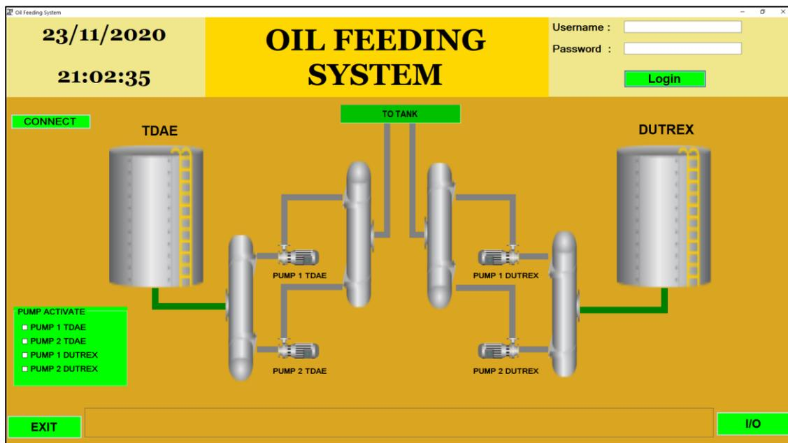
Fig. 9. Main Screen oil feeding system
