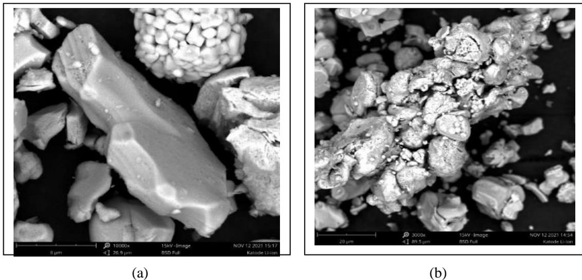
Fig. 4.  $\text{LiCoO}_2$  Surface Morphology: (a) before bioleaching, (b) after bioleaching
