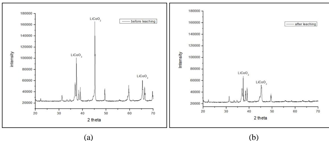
**Fig. 5.** XRD analysis of original LiBs powder of particle size <100 nm. (a) before bioleaching; (b) after bioleaching
