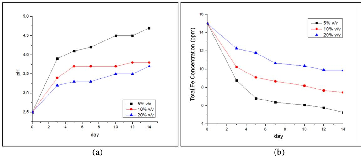
**Fig. 2.** Profile of the activity of *A. ferrooxidans* in terms of (a) pH; (b) Fe<sup>3+</sup> concentration during the bioleaching process of LiBs
