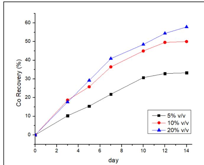
Fig. 3. Cobalt recovery during bioleaching experiment
