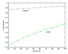
Figure 5. Theoretical dynamic responses of mole fractions of components in the condenser.
