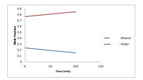
Figure 4. Theoretical dynamic response of mole fraction of component in the reboiler
