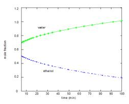
Figure 6. Theoretical Dynamic Responses of Mole Fractions of Components in the Reboiler (Bottom).
