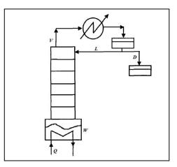
Figure 1. Conventional Batch Distillation Column
