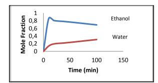
Figure 3. Theoretical dynamic response of mole fraction of component in the condenser
