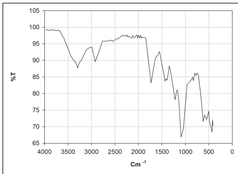
Fig. 1. FTIR spectrum of 2% PVA hydrogel after cross-linking.
