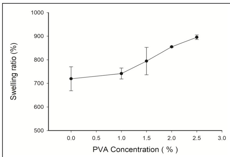
**Fig. 3.** The Effect of PVA Concentration on the Swelling Ratio of the Superabsorbent Hydrogel CMC-Poly(Acrylic Acid)-PVA.
