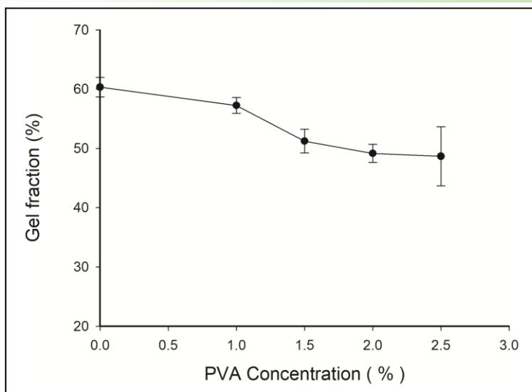
**Fig. 2.** The effect of PVA concentration on the gel fraction of the superabsorbent hydrogel CMC-Poly(Acrylic Acid)-PVA.
