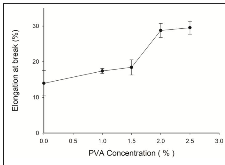
**Fig. 5.** The Effect of PVA Concentration on the Elongation of The Superabsorbent Hydrogel CMC-Poly(Acrylic Acid)-PVA.
