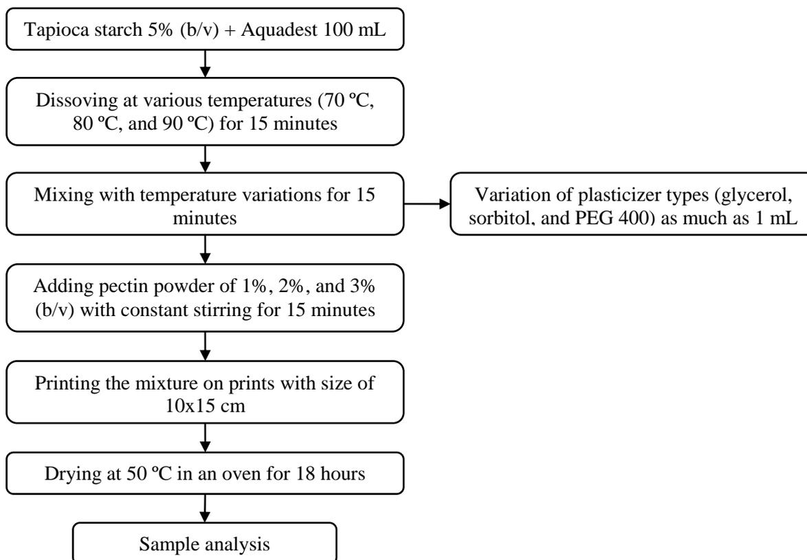
Fig. 3. Schematic procedure of manufacture of edible film.
