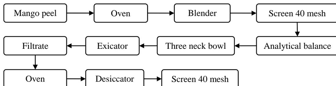
Fig. 2. Scheme of extraction of pectin from mango peel.
