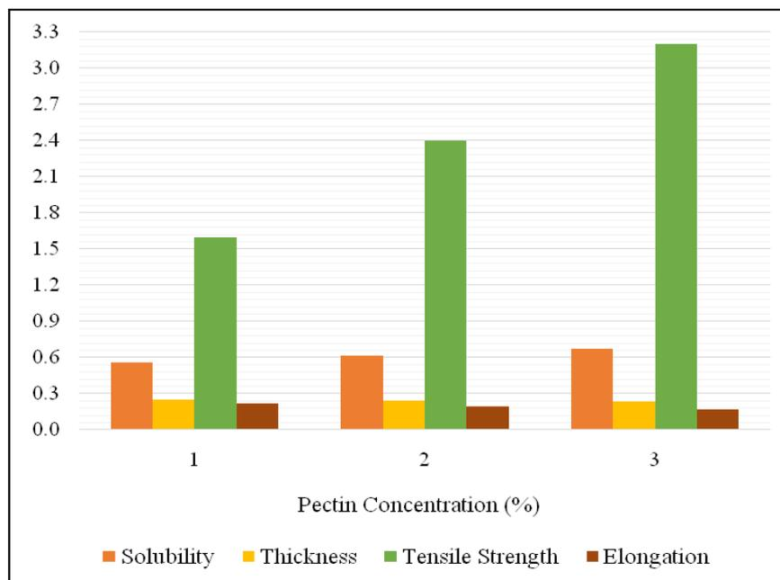
**Fig. 5.** The effect of pectin concentration on the characteristics of edible film.
