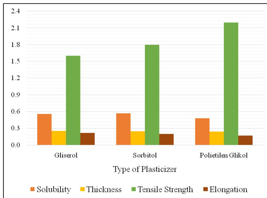
**Fig. 6.** The effect of type of plasticizer on the characteristics of edible film.
