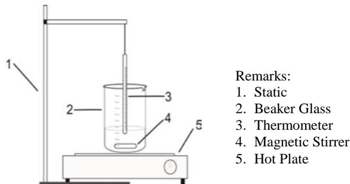
Fig. 1. The main equipment set for manufacturing edible film.
